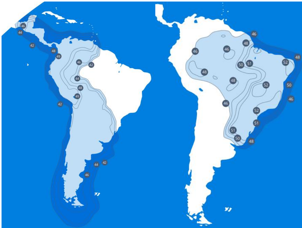
Figure 7: AMZ-5 general America Footprint (Ka (left picture) and Ku (right picture) beams) (Hispasat, Satellite Characteristics AMAZONAS 5)
