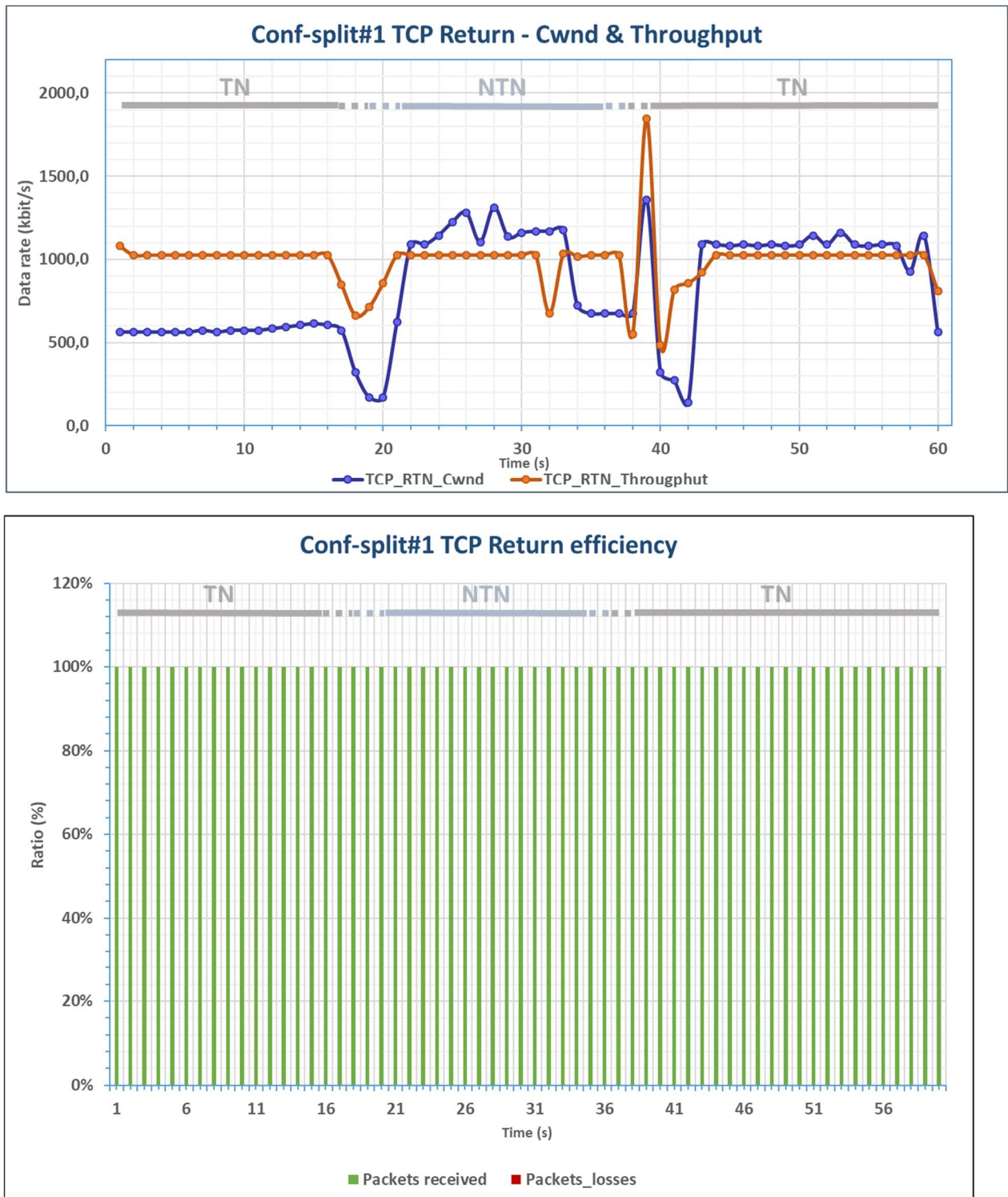
Figure 32: Conf-split#1–TCP RTN Cwnd & throughput data rate-packets transfer measurement graphs
